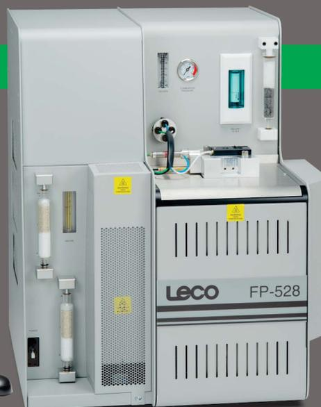
Used specifically for low-sample throughput laboratories, the FP-528 Nitrogen/Protein Determinator is a cost-effective alternative to Kjeldahl digestion methods.
